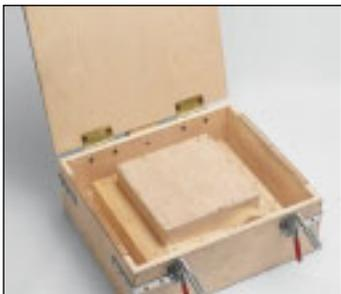
1. A simple wood mold is used to produce the desired cushion shape.
