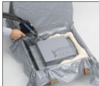
2. Instamate® film is placed into the mold and Instapak® foam is dispensed.
