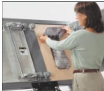
2. When placed into the mold enclosure, an on-board vacuum draws the foam-filled bag into the mold cavity.
