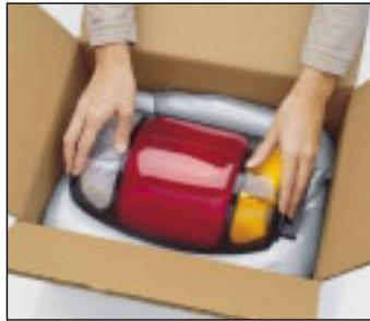
2. The operator places the foam-filled bag into the carton and nestles the product onto the expanding cushion.
