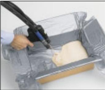
1. Instapak® foam is dispensed into a carton lined with high-strength Instamate® film.
