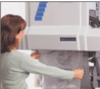
1. With the push of a button, the SpeedyPacker™ system quickly dispenses an Instapak® foam-filled bag.
