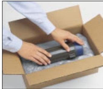
2. The Instamate® film is folded over and the product is placed on the rising foam.
