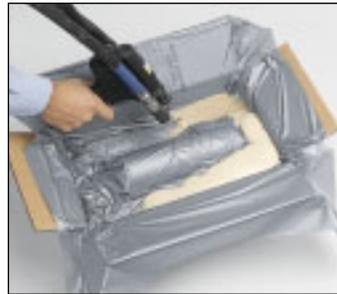
3. A second sheet of Instamate® film is placed over the product and more Instapak® foam is dispensed.
