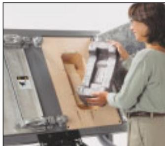
3. Aided by a built-in air ejection system, the operator removes a finished cushion from the mold cavity where it has been allowed to fully expand.
