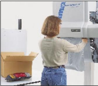
1. At the touch of a button, the operator selects the proper bag length and amount of Instapak® foam required.
