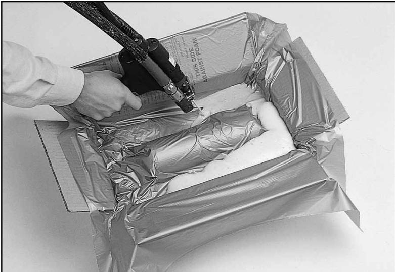
A second sheet of Instamate® packaging film is placed over the item, and more Instapak® foam is dispensed.
