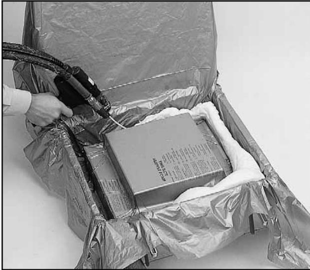
Instamate® packaging film is placed into the mold and Instapak® foam is dispensed into the mold cavity. The film is folded over the rising foam. Make sure enough film is used to cover the lid of the mold. Close the lid. The foam rises into the proper shape, and the cushion is removed.
