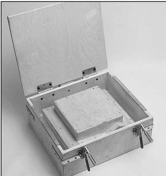
A simple wood mold is used to produce the desired cushion shape.
