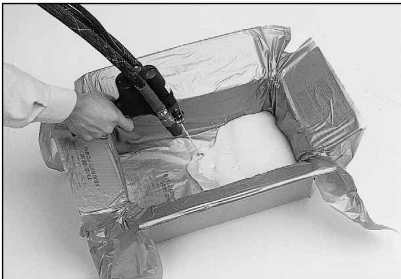
Instapak® foam is dispensed into a carton lined with high strength Instamate® packaging film.
