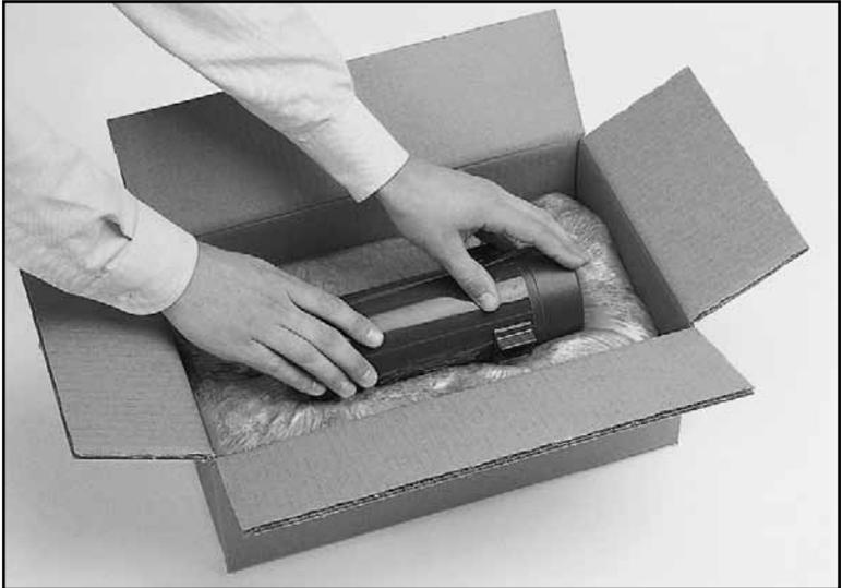
The Instamate® packaging film is folded over and the item to be packaged is placed on top of the rising foam.
